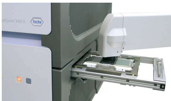
Figure 19: Automated LightCycler® 480 Instrument loading process.
